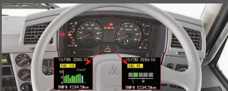
The new dash has a colour display that shows important information such as average and current fuel consumption, oil level and service replacement requirements.
