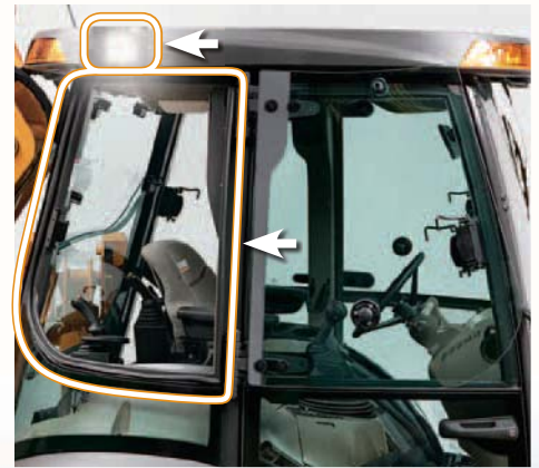
New rear-quarter windows and side lighting
